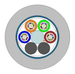
**Central strength member (CSM):** glass fibre reinforced plastic rod
